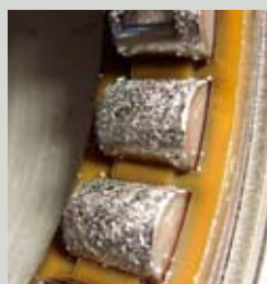
Roller bearing failure
