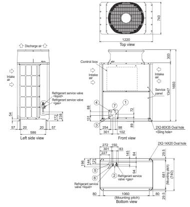
net . Please refer to me Installation Manual for information regarding necessary spacing around the unit and foundation work.
