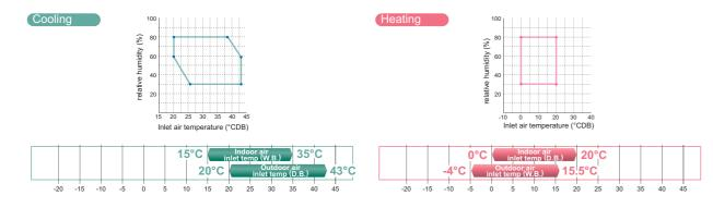
Heating operation is available at -4°C Outdoor temperature making it adaptable for places with frequent heating requirements.
