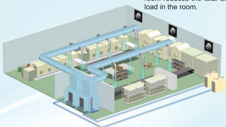
\*1 Fresh air intake type indoor units supply pretreated outside air into the room. This type of units are not designed to handle internal thermal load. Use other types of air conditioning units that are capable of handling internal thermal load in combination with the Fresh Air Intake type units.
