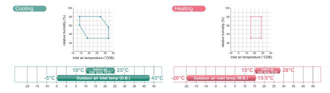
By controlling the air volume of the outdoor unit fan, operation is available even when the outdoor temperature is -5°C for cooling and -20°C for heating.
