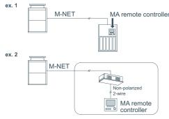
\*When a PAR-31MAAE is connected to a group, no other MA remote controllers can be connected to the same group.
